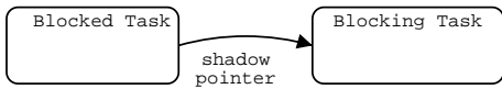
Figure 1. The shadow relationship can be thought as a pointer to a shadow task.
