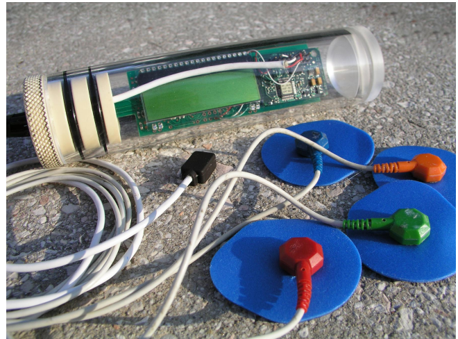
Fig. 6. First prototype in a Lexan housing
