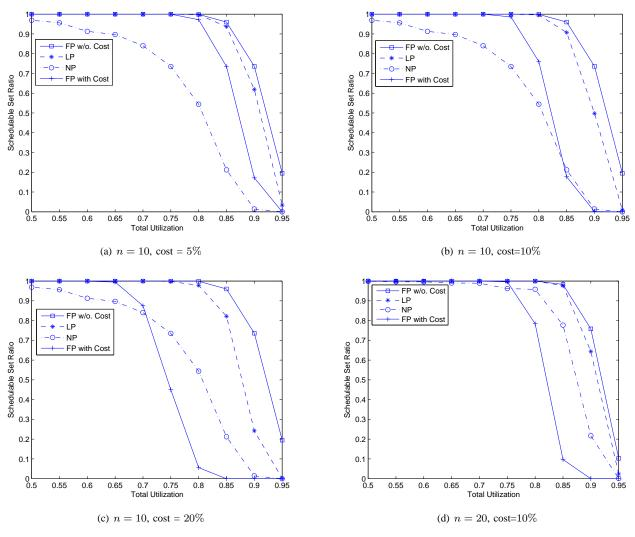
Figure 5. Percentage of schedulable task sets varying n and the preemption cost.
