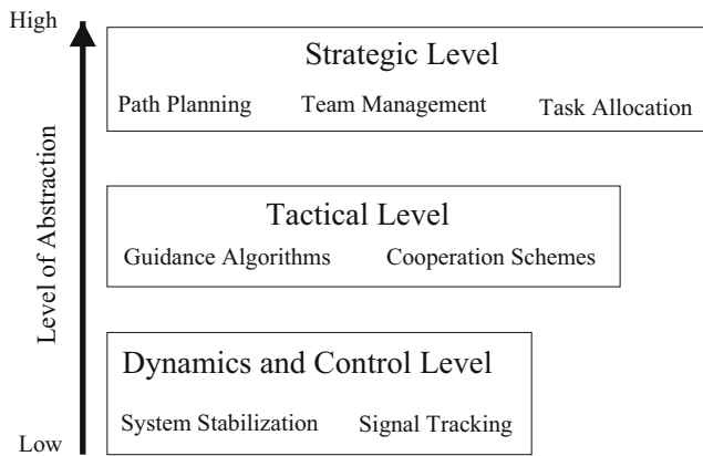
Fig. 1 Abstraction levels in the development of applications involving autonomous vehicles
