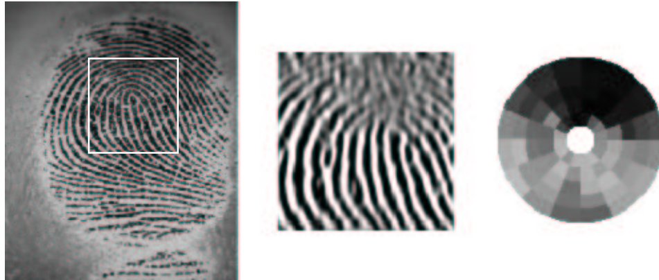
Figure 26: Example of Fingercode computation: a region of interest is determined around the core, then it is directionally filtered (only vertical filtering is showed), tessellated and intensity absolute deviations (represented in gray scale) are computed.
