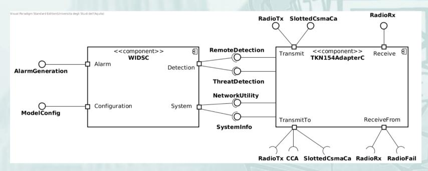
Realized a TinyOS component integrated with 802.15.4 stack
