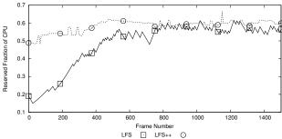
**Figure 13.** Inter-Frame times and reserved fraction of CPU time for mplayer when LFS and LFS++ are used.
