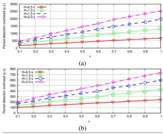
**Figure 8.** Period detection overhead, as a function of the observation time H and the  $\epsilon$  parameter.
