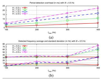
**Figure 7.** Time to compute the frequency transform (top), and corresponding precision in frequency detection (bottom), as a function of the observation time H and  $f_{max}$ , at fixed  $\delta f = 0.5Hz$  and  $\epsilon = 0.5Hz$ .
