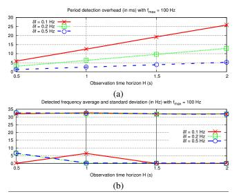
**Figure 6.** Time to compute the frequency transform (top), and corresponding precision in frequency detection (bottom), as a function of the observation time H and  $\delta f$ , at fixed  $f_{max}=100Hz$  and  $\epsilon=0.5Hz$ .
