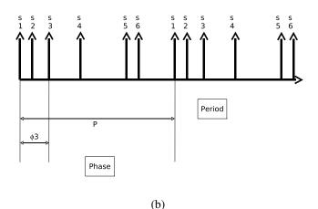
**Figure 5.** A) a sequence of events associated to a segment of execution of an application, B) The mathematical model as a sequence of Dirac Deltas  $(\delta)$ .
