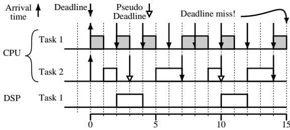
**Figure 8. Also EDF with modified deadlines does not work always.**
