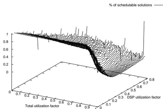
**Figure 15. Difference in the percentage of scheduled tasks set between our approach and DPCP when considering the influence of DSP utilization.**
