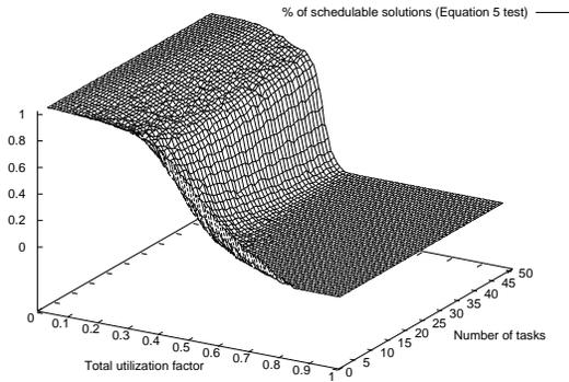
**Figure 10. Schedulability results of DPCP when varying the total utilization factor and the number of tasks in the task set (using Equation (4) ).**
