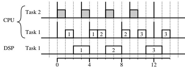
Figure 3. A task set that cannot be feasibly scheduled by RM and EDF (jobs of task  $\tau_1$  are numbered to facilitate interpretation): task  $\tau_1$  misses all its deadlines.
