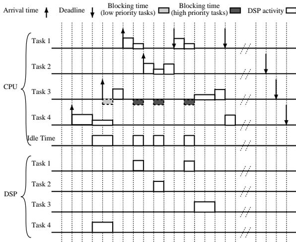
**Figure 6. Example of scenario where task  $\tau_3$  is blocked by some high priority ( $\tau_1$  and  $\tau_2$ ) and low priority ( $\tau_4$ ) tasks.**
