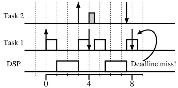
**Figure 7. EDF does not work always.**
