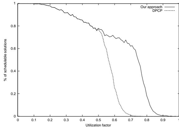
**Figure 14. Performance of the two approaches and their difference as a function of the utilization factor for task sets composed by 30 tasks.**
