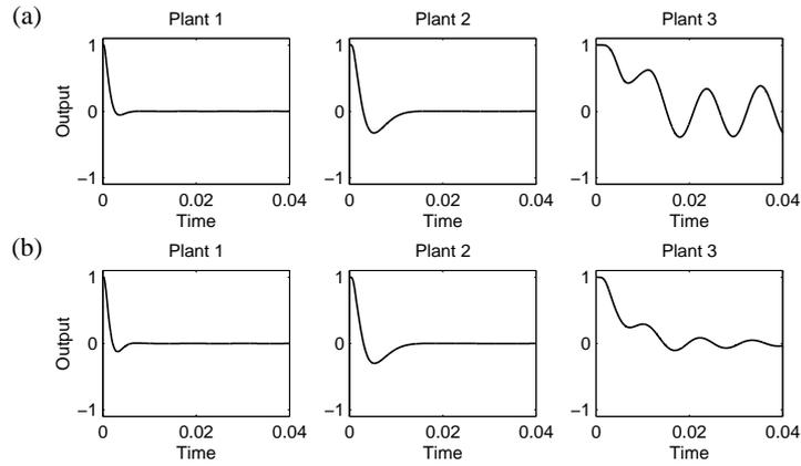
**Fig. 7.** Control system responses under EDF scheduling: (a) after one iteration, (b) after ten iterations.
