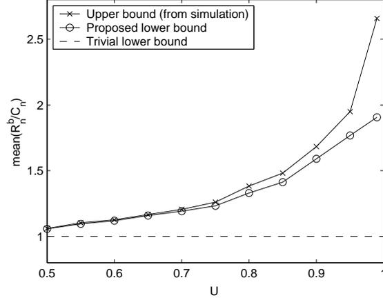
**Fig. 4.** Comparison of bounds on the best-case response time under EDF. The results are shown for the longest-period task.
