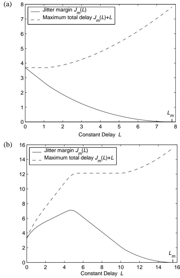
**Fig. 3.** Example of jitter margins  $J_m(L)$ : (a) PID controller with  $h = 10$ , (b) LQG controller with  $h = 10$ , designed for the delay  $L = 5$ . (All units are in ms.)
