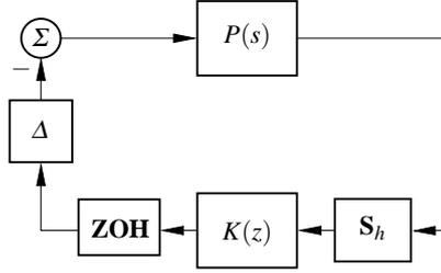
**Fig. 1.** Computer-controlled system with continuous-time plant  $P(s)$ , periodic sampler  $S_h$ , discrete-time controller  $K(z)$ , zero-order hold, and time-varying delay  $\Delta$ .
