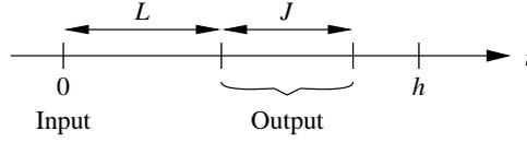
**Fig. 2.** The input-output delay can be divided into a constant delay,  $L$ , and a jitter,  $J$ .
