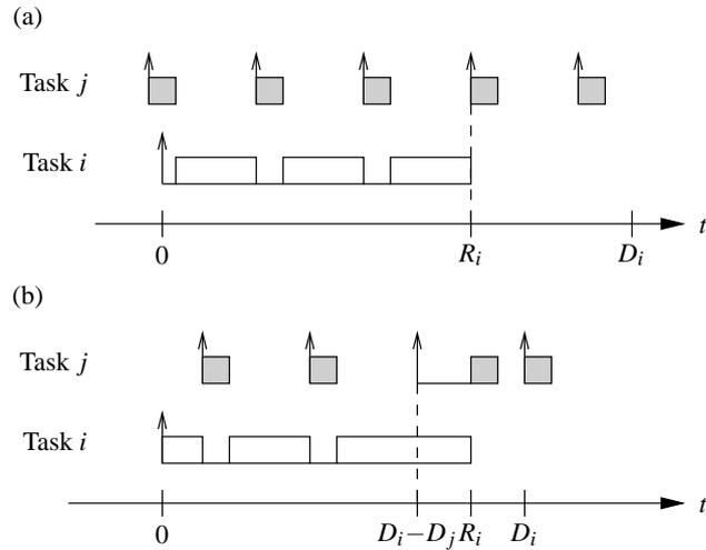
**Fig. 8.** Different cases where task *j* causes minimum interference for task *i*: (a)  $D_i - D_j > R_i$ , (b)  $D_i - D_j \leq R_i$ .
