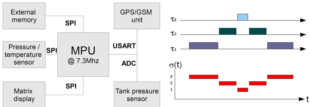
**Figure 1 a) Hardware diagram**
