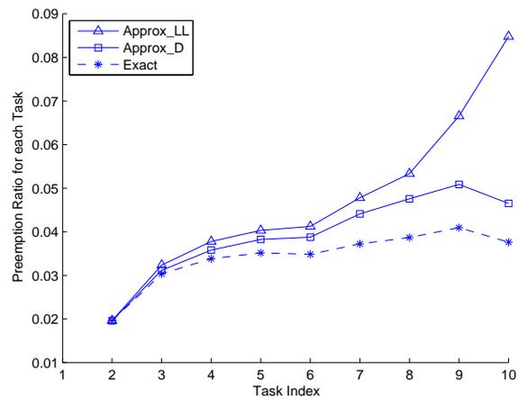
Figure 5. Average preemption ratios for each task when  $D = T$  and  $U_{tot} = 0.7$ .
