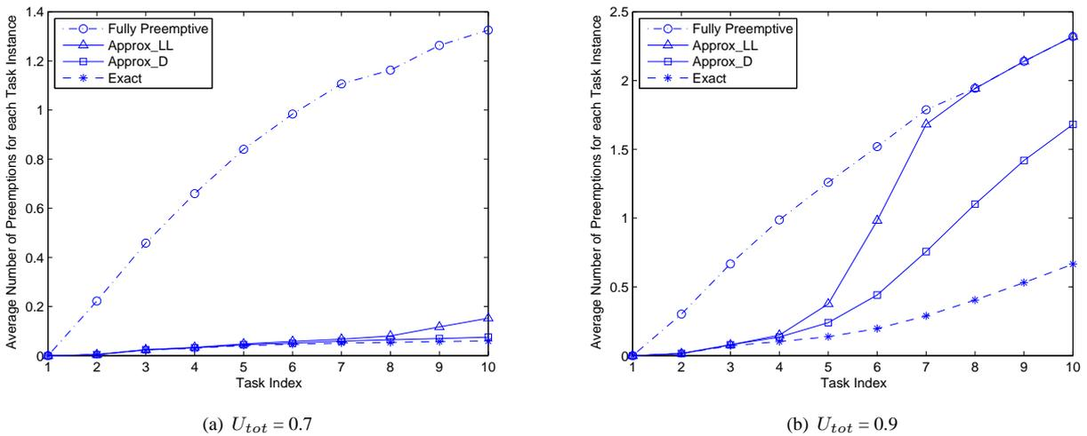
Figure 7. Average number of preemptions for each task instance when  $D = T$ .
