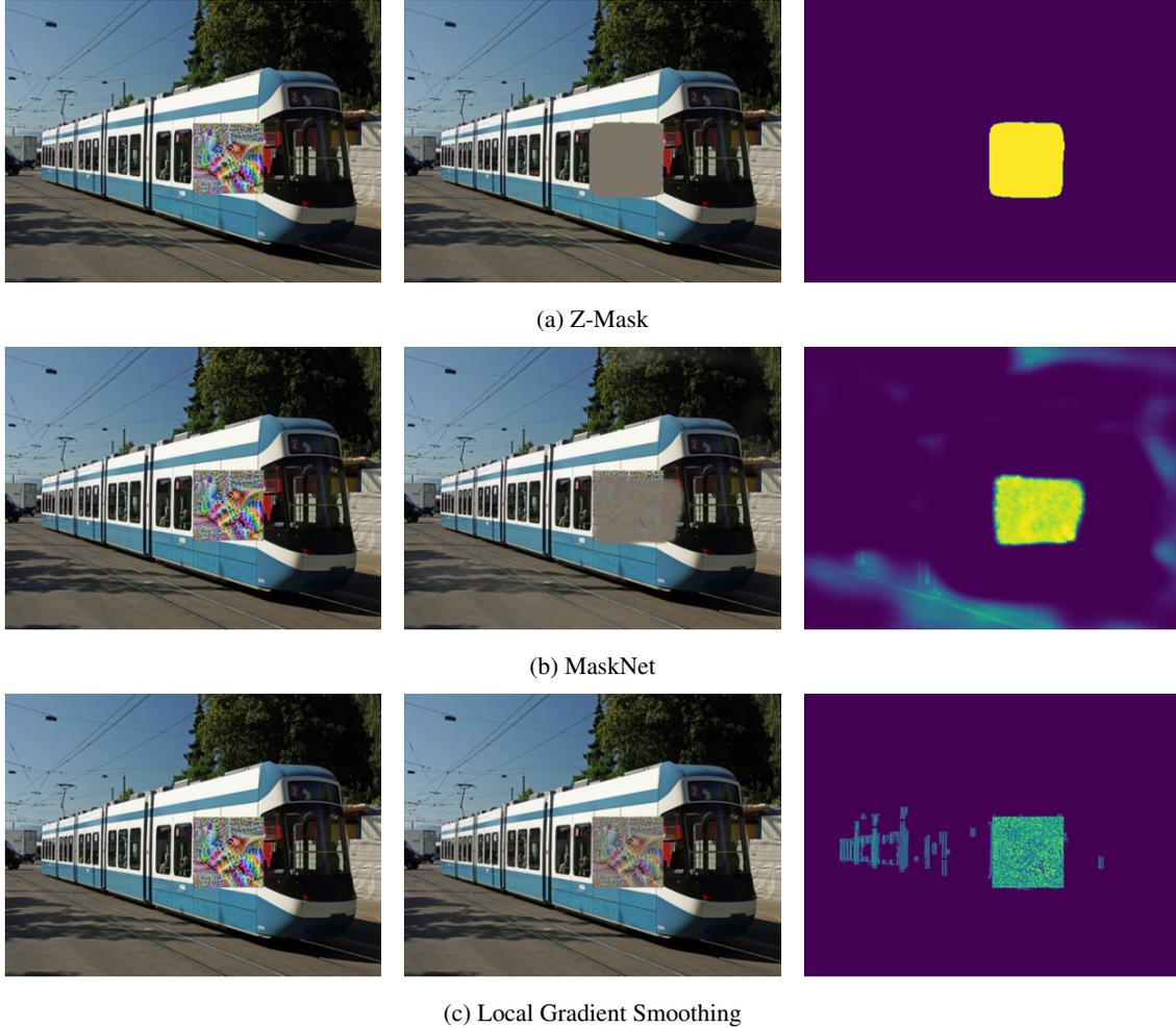
Figure 12: Comparison of the masks obtained with different methods: (a) *Z-mask*, (b) MaskNet, and (c) LGS.
