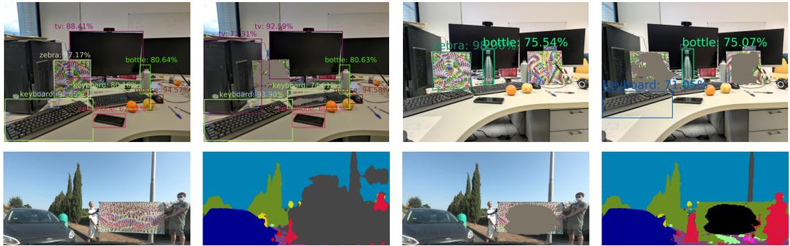
Figure 8: Examples of the masking effects on physical attacks for object detection (on RetinaNet) and semantic segmentation (on ICNet). A defense mask not only protects the model by removing wrong local adversarial predictions associated with the patch, but also mitigates its global effects in corrupting other objects in the image.
