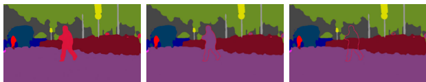
Fig. 3. Illustration of how the original label (left) can be modified to attack the class pedestrian : by changing pedestrian with road class (middle), or using the nearest neighbor approach (right).
