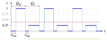
$$s_{eq} = \frac{s_{H}(Q_{H} - o_{LH}) + s_{L}(Q_{L} - o_{HL})}{Q_{H} + Q_{L}}$$
