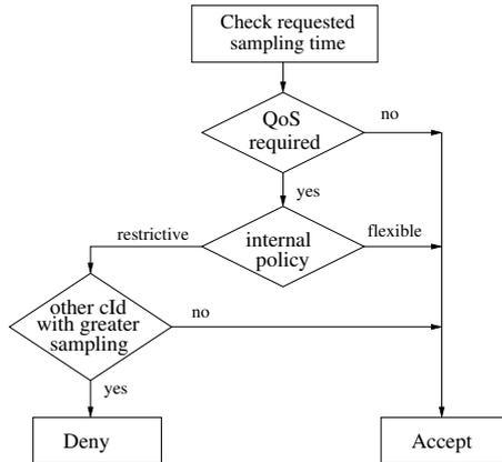
Figure 4. Access control module
