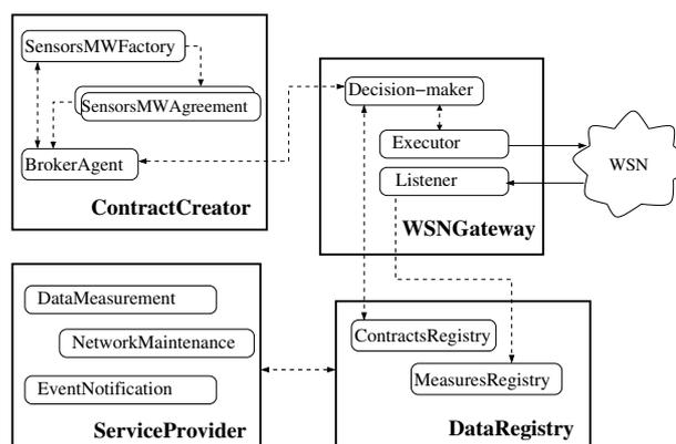
**Figure 2. SensorsMW architecture**
