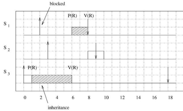
Fig. 1. In this example, blocking times are not correctly accounted for.
