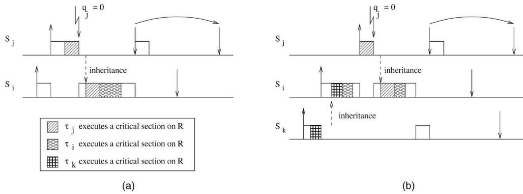
Fig. 3. Example of blocking situations with SRT tasks: (a) An SRT task with a short period blocks an HRT task with a long period. (b) An HRT task is blocked twice on resource R.
