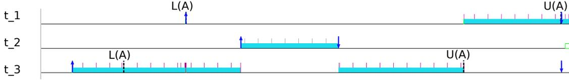
**FIGURE 4:** Two task ( $\tau_1$  and  $\tau_3$ ) sharing one resource (protected by a normal mutex). A third independent task ( $\tau_2$ ) arrives and preempts  $\tau_3$  even if  $\tau_1$ 's server has higher priority than  $\tau_2$ 's.
