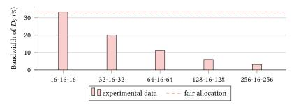
Fig. 2. Percentage of the bandwidth used by  $D_2$  as a function of the burst size of  $D_1$  and  $D_3$ . The labels below each pair of bars indicate the burst size of  $D_1$ ,  $D_2$  and  $D_3$ , respectively.
