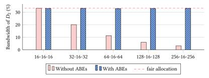
Fig. 11. Percentage of the total bandwidth used by  $D_2$  as a function of the burst size of  $D_1$  and  $D_3$ . The labels below each pair of bars indicate the burst size of  $D_1$ ,  $D_2$  and  $D_3$ , respectively.
