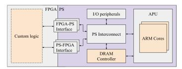
Fig. 1. Simplified architecture of a SoC FPGA platform.
