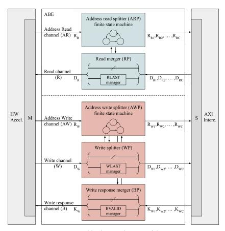
Fig. 9. Internal hardware architecture of the ABE.
