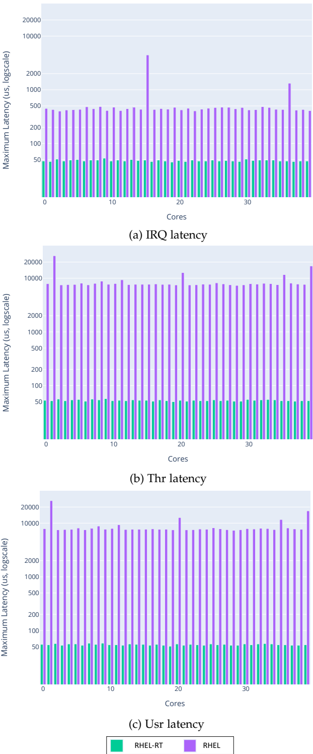
Fig. 15: Bar chart of the maximum latency values (logscale) obtained by running Timerlat for 6 hours in the workload configuration on 40 cores running RHEL (in violet) and RHEL-RT (in green).
