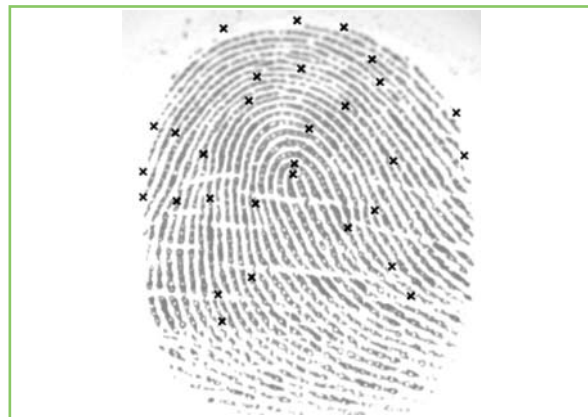
Figure 1 - Example of minutiae detection. Some false minutiae have been detected on the image border.
