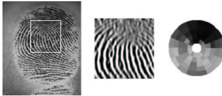
Figure 1. Example of Fingercode computation: a region of interest is determined around the core, then it is directionally filtered (only vertical filtering is showed), tessellated and intensity absolute deviations (represented in gray scale) are computed.
