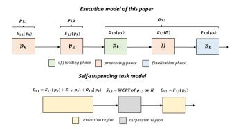
**Figure 4:** Example mapping of the model proposed in this paper to the self-suspending task model for analysis purpose.
