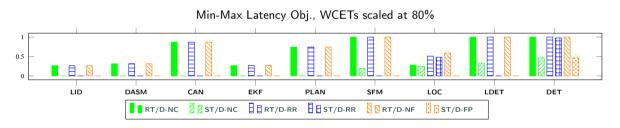
**Figure 8:** Ratio between the obtained WCRT bounds and the deadline, and the suspension time bounds and the deadline for each task of the WATERS 2019 Challenge obtained by running the MILP with the Min-Max Latency objective function and WCET scaled at the 80% of their values.
