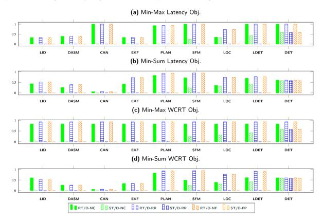
Figure 7: Ratio between the obtained WCRT bounds and the deadline, and the suspension time bounds and the deadline for each task of the WATERS 2019 Challenge obtained by running the MILP with different objective functions reported above each graph.
